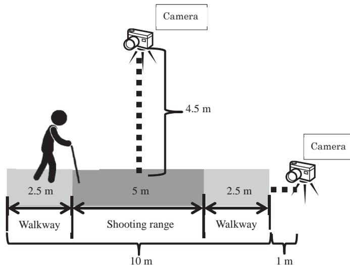
Fig. 1 Setting of walkway and digital cameras for measurement
